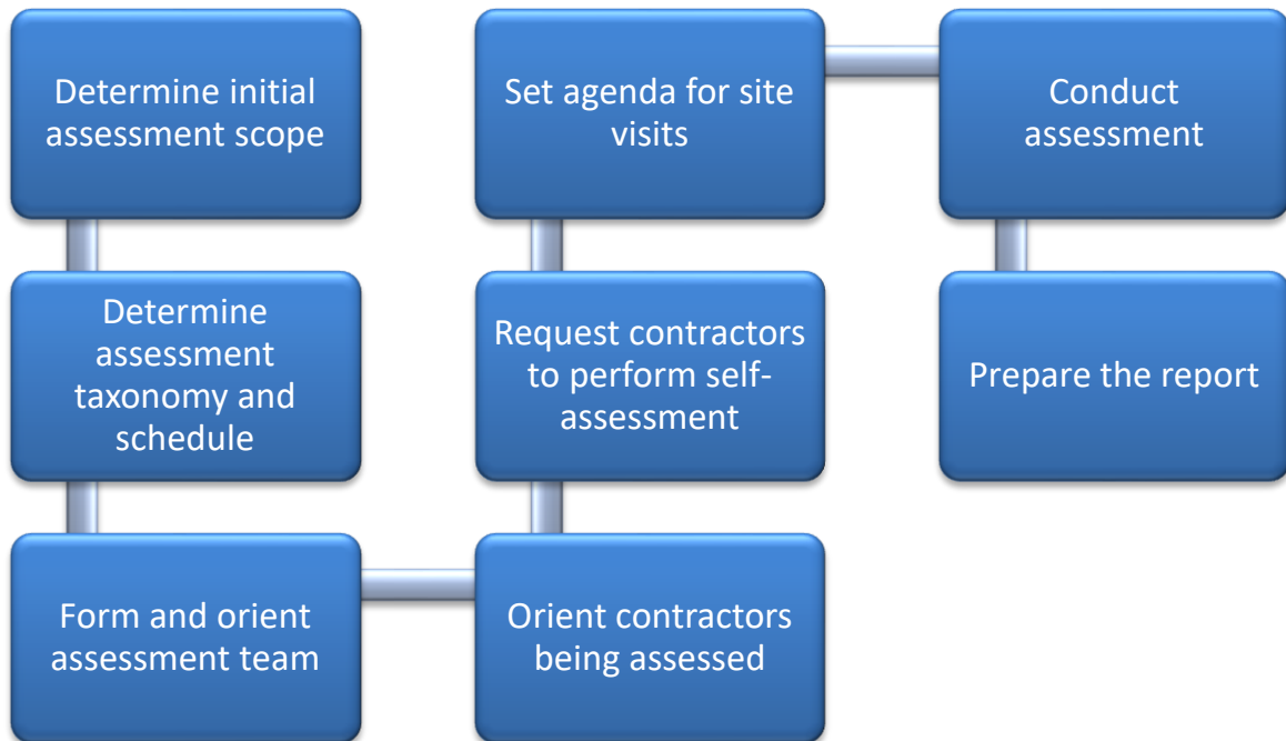
Figure 4-1 Sample Process Flow for Conducting an Assessment of Manufacturing Readiness
